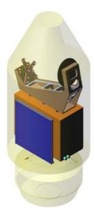
Figure 5.52. Accommodation of SKIM in the Vega-C fairing on top of short VESPA-C, Concept A (left) and Concept B (right).
